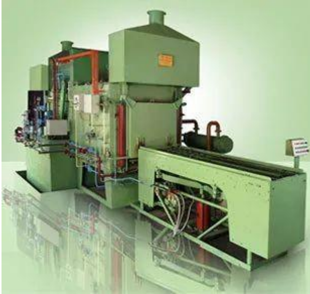
Sealed Quench Furnace - 2 Nos. (650 Kgs)
