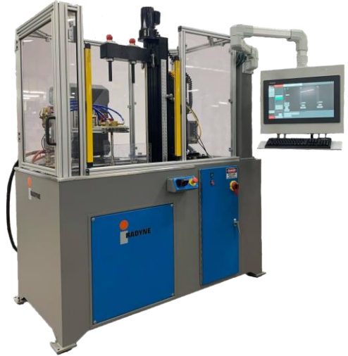
Induction Hardening Machine - 2 Nos. (with scanning, high freq.)
